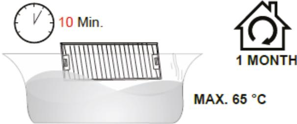
3. Clean with a soft cloth/brush. Rinse thoroughly and dry well. The filter can be cleaned in the dishwasher.
